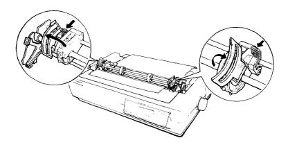
5. Adjust the sprocket units to match the width of the paper and adjust the paper supports so they are evenly placed between the sprocket units.
